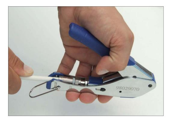
1. Insert the cable with the mounted CX3 connector as shown above
