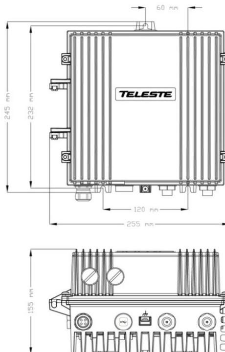
Figure 1. AC8810 housing dimensions – top and side view
