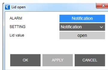
Figure 18. The discrete alarm configuration dialog box
