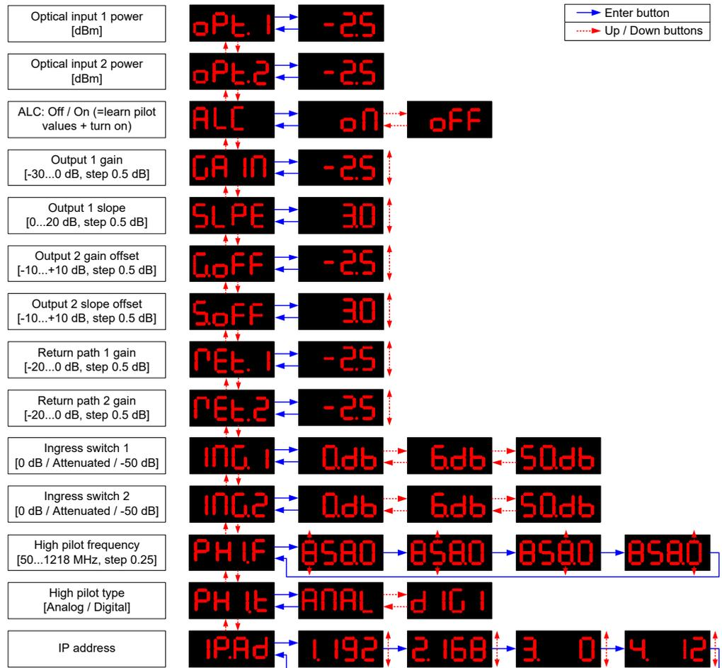
Turning on ALC via the local UI performs two tasks: 1) copies the measured pilot levels to target levels and 2) enables ALC.
