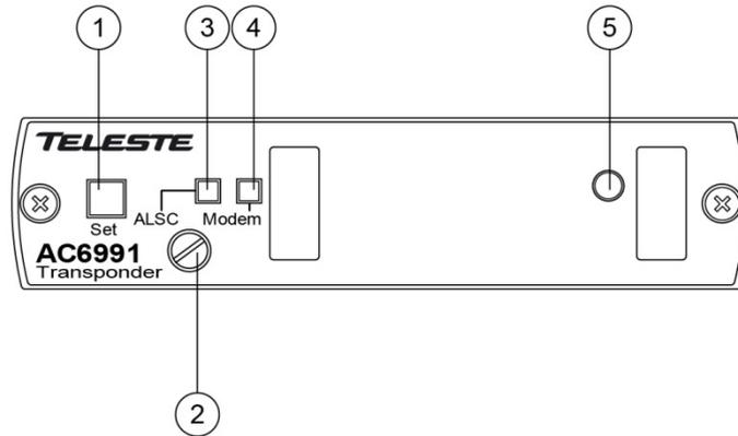
Figure 4. AC6991 transponder unit, 1) "Set" -button, 2) Fastening bolt, 3) Indicator for ALSC status, 4) Indicator for modem status, 5) Light sensor
