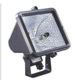
Multifunctional floodlights in die-cast aluminium, painted with polyester powders, for fixed applications. Optic in 99.85% polished and anodised aluminium. Flat tempered glass 5mm thickness. Anti-aging silicone gasket. Suitable for use with halogen lamps. Power input through cable gland for cable  $\emptyset$  9÷12 mm.
